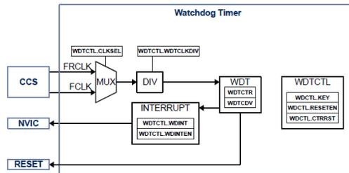
The WDT is a 24-bit count-down timer. This timer may be configured to be clocked either from the FRCLK (input to the PLL) or FCLK (output of the PLL). Because of this, this timer may be used as a wakeup timer when the ARM Cortex-M0 is in deep sleep mode.
