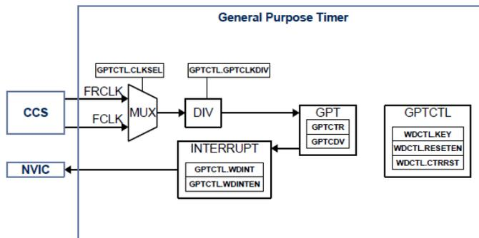
The GP Timer is a 24-bit count-down timer. This timer may be configured to be clocked either from the FRCLK (input to the PLL) or FCLK (output of the PLL). Because of this, this timer may be used as a wakeup timer when the ARM Cortex-M0 is in deep sleep mode.
